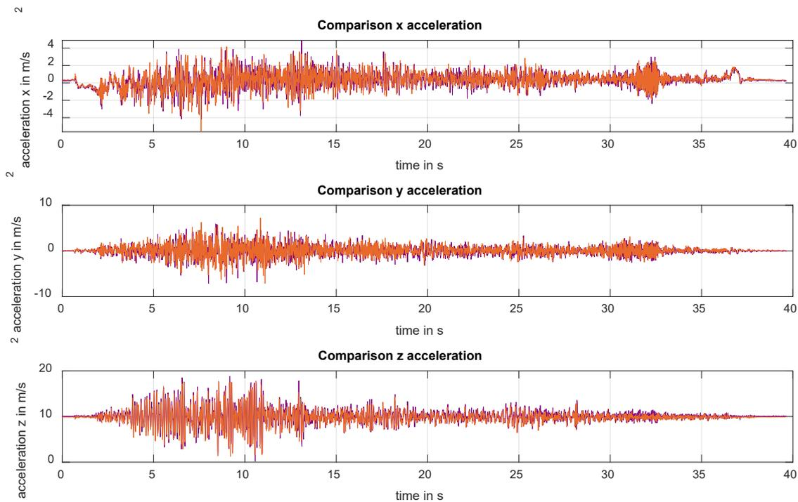
Figure 8: Comparison of all acceleration data of test run 03\_Rollout\_01 (purple: MPU-9150; orange: LPMS-CU2)
