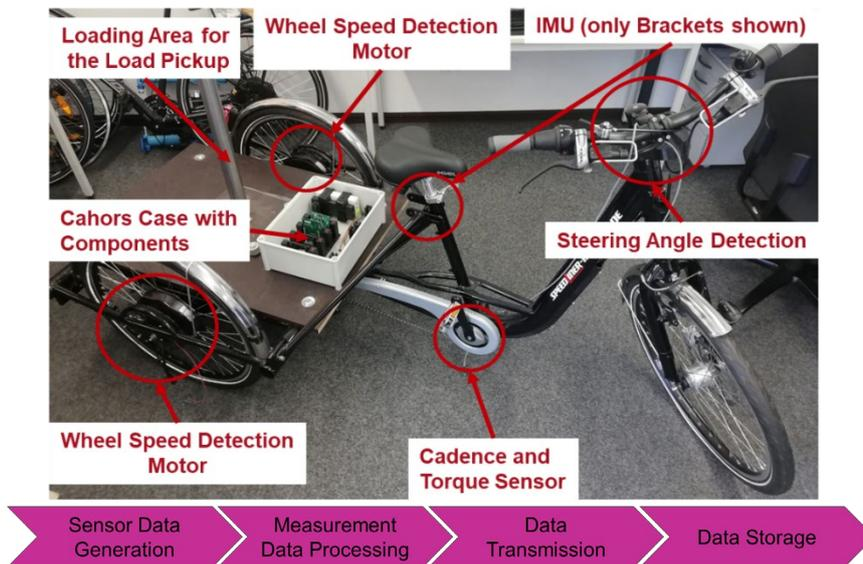
Figure 1: Peripheral overview and data-processing concept
