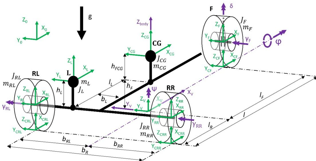
Figure 7: Integrated vehicle and calculation models in the simulation model [2]
