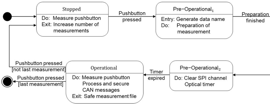
Figure 3: State diagram of the data logger
