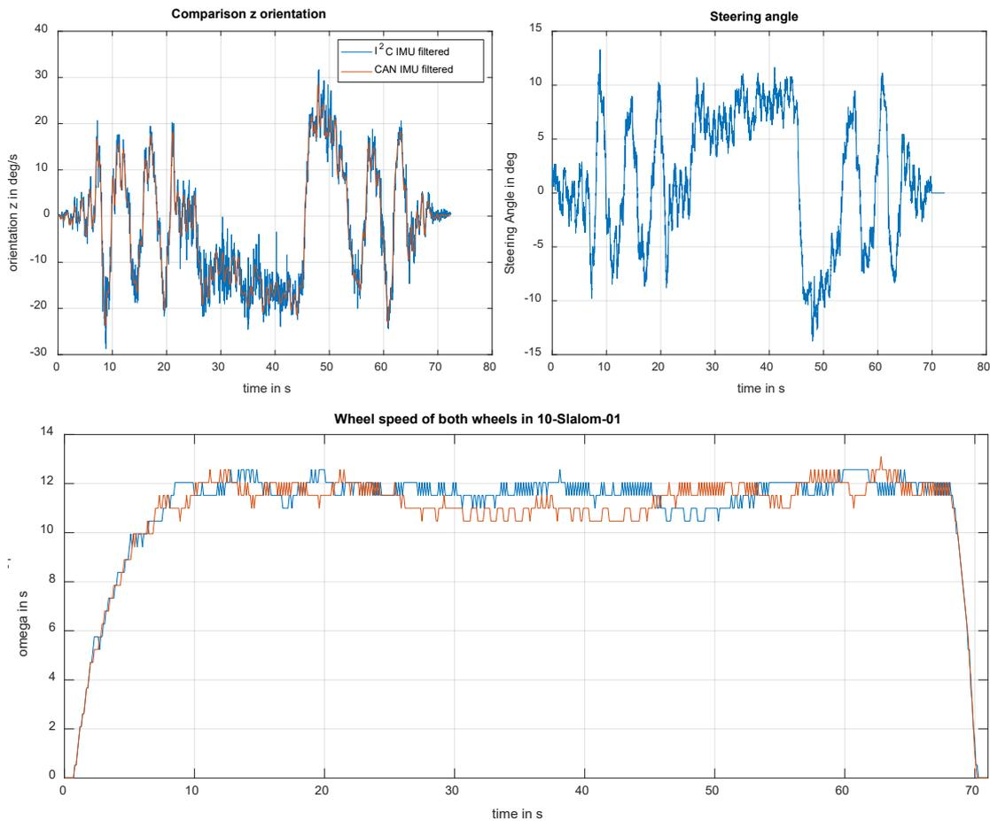
Figure 9: Overview of the slalom track test: comparison of the IMUs z orientation (Left top), measurement results of the steering angle (Right top), measurement results of both wheel frequencies (Bottom)
