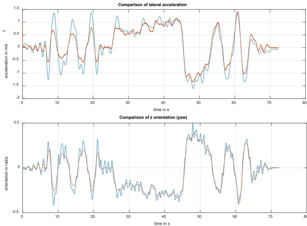
Figure 12: Comparison of lateral acceleration and z-orientation in measurement 10\_Slalom\_01 (blue: measurement; orange: simulation)
