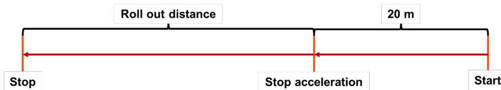
Figure 4: Test scenario "roll out"
