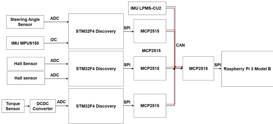
Figure 2: Sketch of the hardware structure
