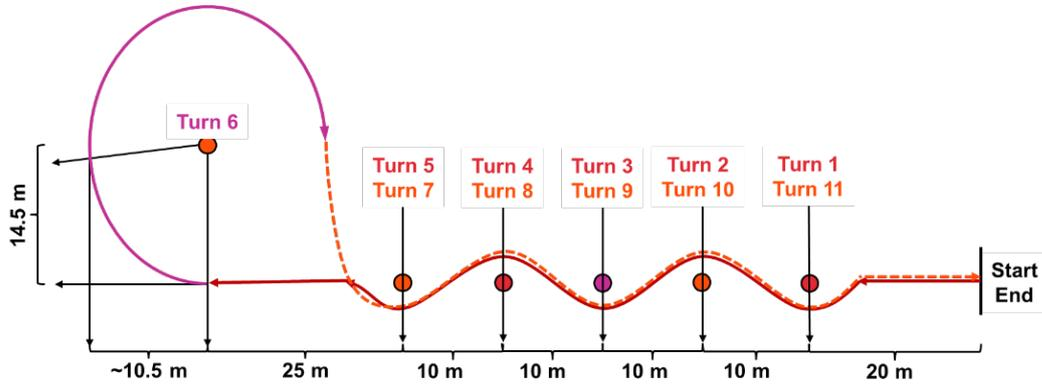
Figure 6: Test scenario “slalom track”
