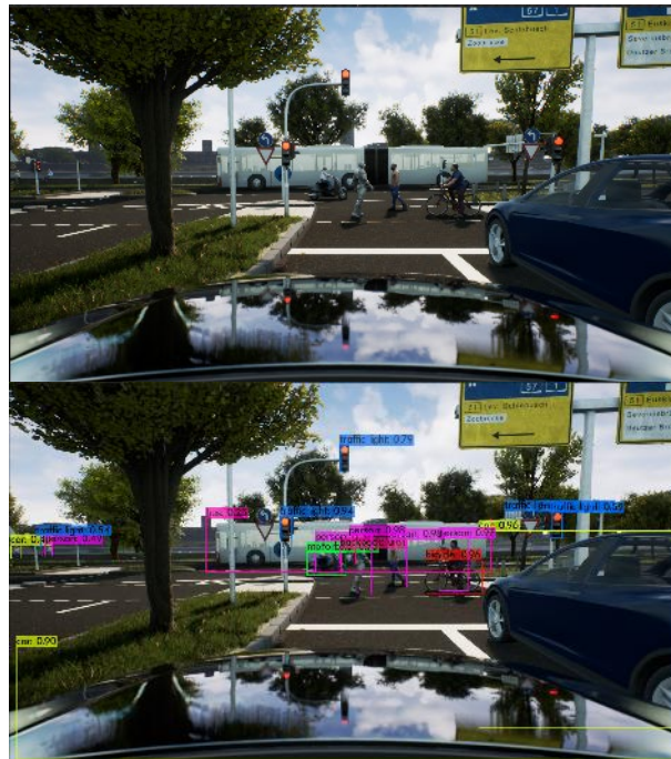
Figure 26: Results of the AI-based camera model, without and with recognized objects
