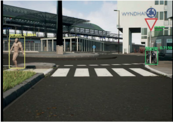
Figure 8: Pedestrian crossing scene. Left: YOLO-algorithm result. Right: MobileEye setup.
